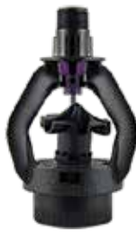
Model 615 (black) 6-groove 15° trajectory Large droplets Nozzle sizes #10-24
